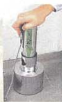
Rebound Hammer Test – Measure the surface hardness of the concrete 利用回彈測試—量度表面混凝土硬度
