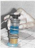
Half-cell Potential Measurement on the concrete. 利用半電池電壓及電阻測試 勘察混凝土內的鋼筋生銹度
