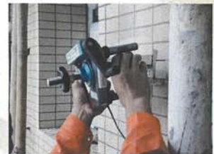
Bond Test – Measure the adhesive strength and the tensile strength of the overlay 利用黏著力測試—量度覆蓋料的黏著力表面抗拉力
