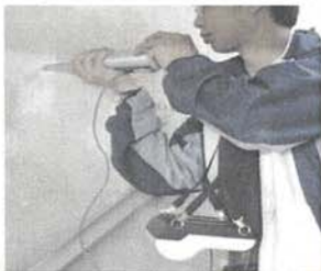
Rebound Hammer Test – Measure the surface hardness of the concrete 利用回彈測試—量度表面混凝土硬度
